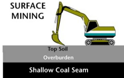
**Surface mining** is used to produce most of the coal in the U.S. because it is less expensive than underground mining. Surface mining can be used when the coal is buried less than 200 feet underground. In surface mining, giant machines remove the top-soil and layers of rock to expose large beds of coal. Once the mining is finished, the dirt and rock are returned to the pit, the topsoil is replaced, and the area is replanted. The
