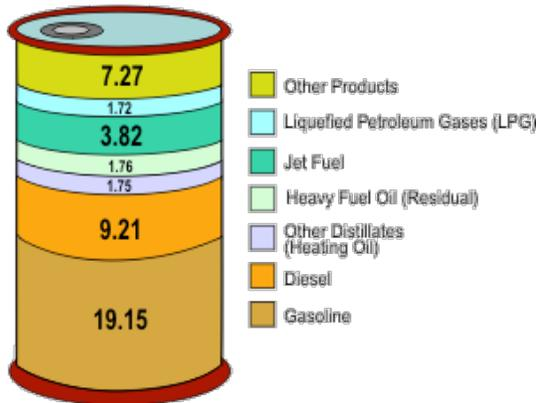
After crude oil is removed from the ground, it is sent to a [refinery](#) by pipeline, ship or barge. At a [refinery](#), different parts of the crude oil are separated into useable petroleum products. Crude oil is measured in barrels (abbreviated "bbls"). A [42-U.S. gallon barrel](#) of crude oil provides slightly more than 44 gallons of petroleum products. This gain from processing the crude oil is similar to what happens to popcorn, it gets bigger after it is popped.
