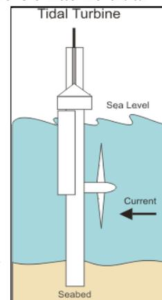
Tidal turbines are a new technology that can be used in many tidal areas. They are basically wind turbines that can be located anywhere there is strong tidal flow. Because water is about 800 times denser than air, tidal turbines will have to be much sturdier than wind turbines. They will be heavier and more expensive to build but will be able to capture more energy.
